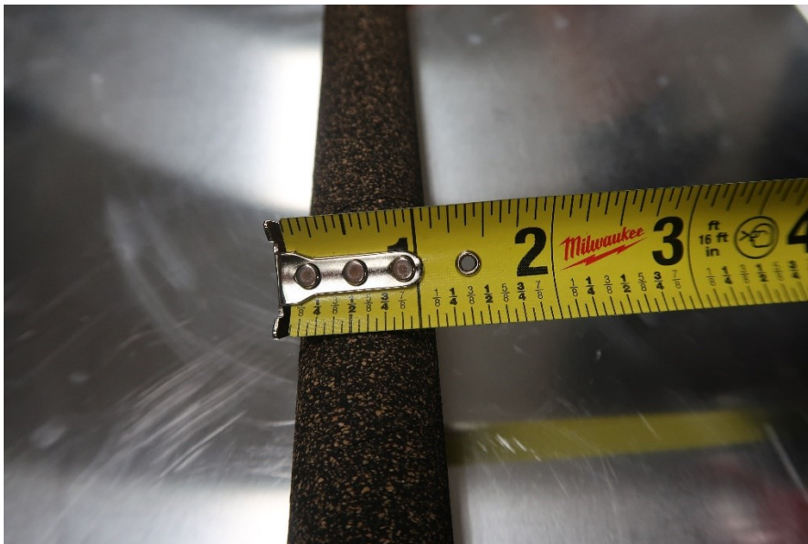
Medium Diameter Rod (Calstar GFGR 800M) Use standard clamp
