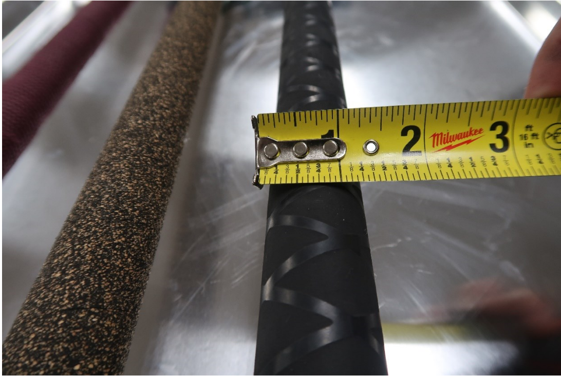
Large Diameter Rod (Super Seeker 6480 CT) Use Large Clamp size
